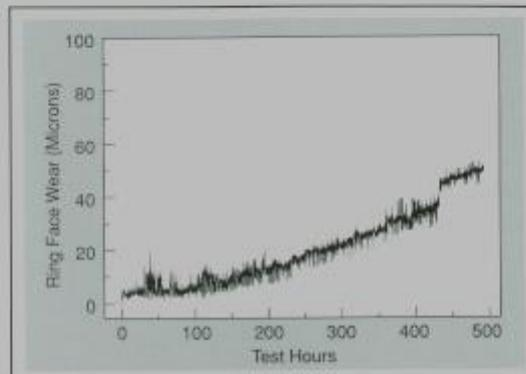
Piston ring wear is measured using the SLA technique.
