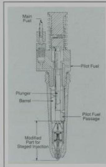
Experimental staged injectors are used for low cetane number fuels.
