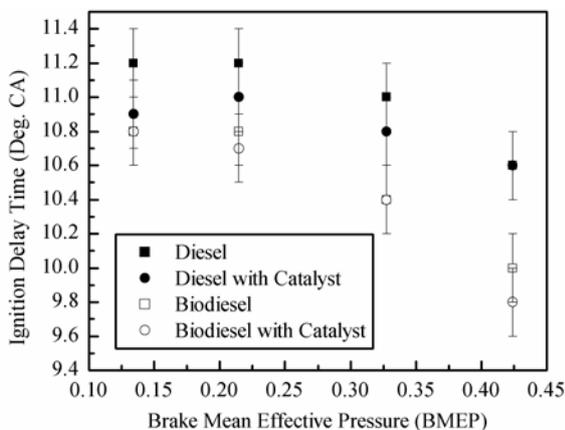
Figure 7 The ignition delay time as a function of the engine load (BMEP) for the tested four fuels
