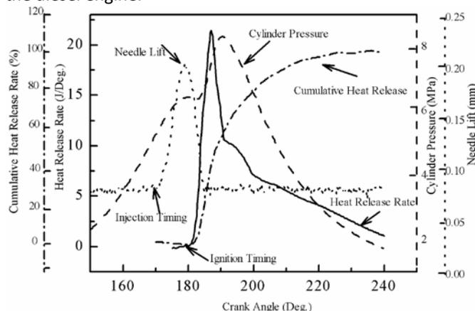
Figure 2 Definitions of combustion characteristics in diesel engines
