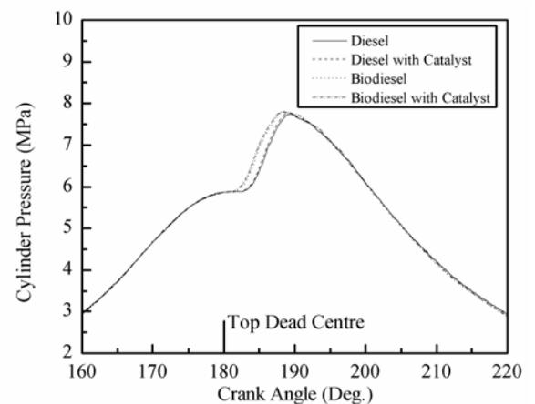
Figure 5 In-cylinder pressure for both diesel and biodiesel dosed with and without the catalyst under engine speed 3200rpm and engine load 0.33MPa
