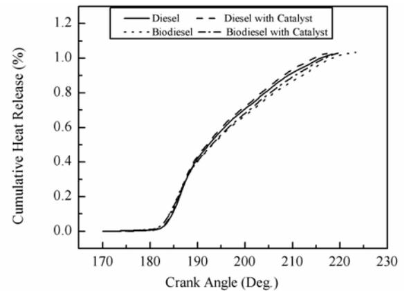
Figure 8 cumulative heat release for both diesel and biodiesel dosed with and without the catalyst under engine speed 3200rpm and engine load 0.33MPa
