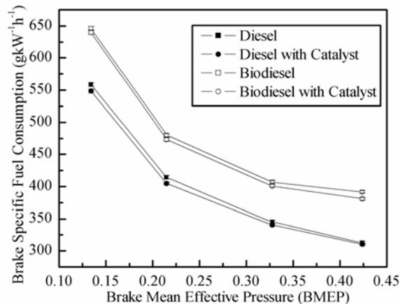
Figure 3 The brake specific fuel consumption as a function of the engine load (BMEP)
