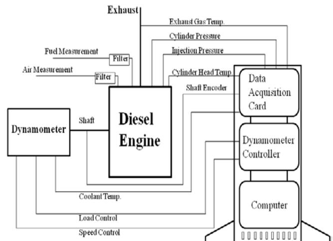
Figure 1 A schematic diagram of the diesel engine test bench
