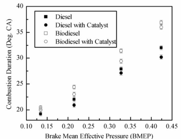
Figure 9 The combustion duration as a function of the engine load (BMEP) for the tested four fuels
