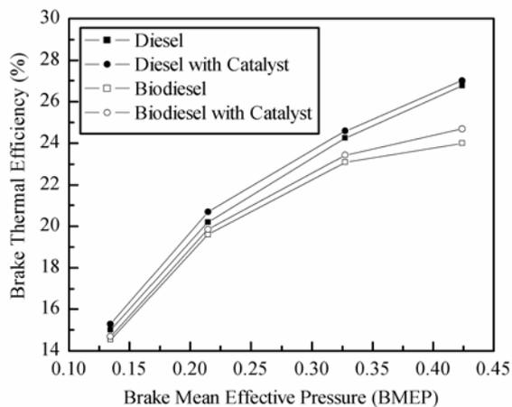
Figure 4 The brake thermal efficiency as a function of the engine load (BMEP)
