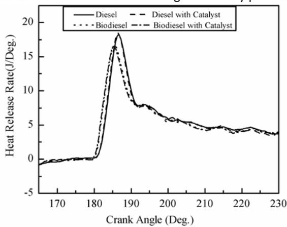
Figure 6 heat release rate and cumulative heat release for both diesel and biodiesel dosed with and without the catalyst under engine speed 3200rpm and engine load 0.33MPa
